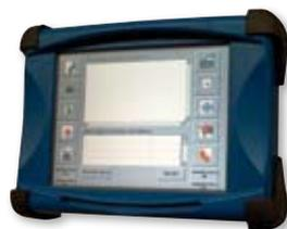
Among the available accessories, the touch screen MDT4000 allowing for a better management of messages and alarms as well as mobile office applications based on Windows XP, NT embedded, Windows CE.net or LINUX.
